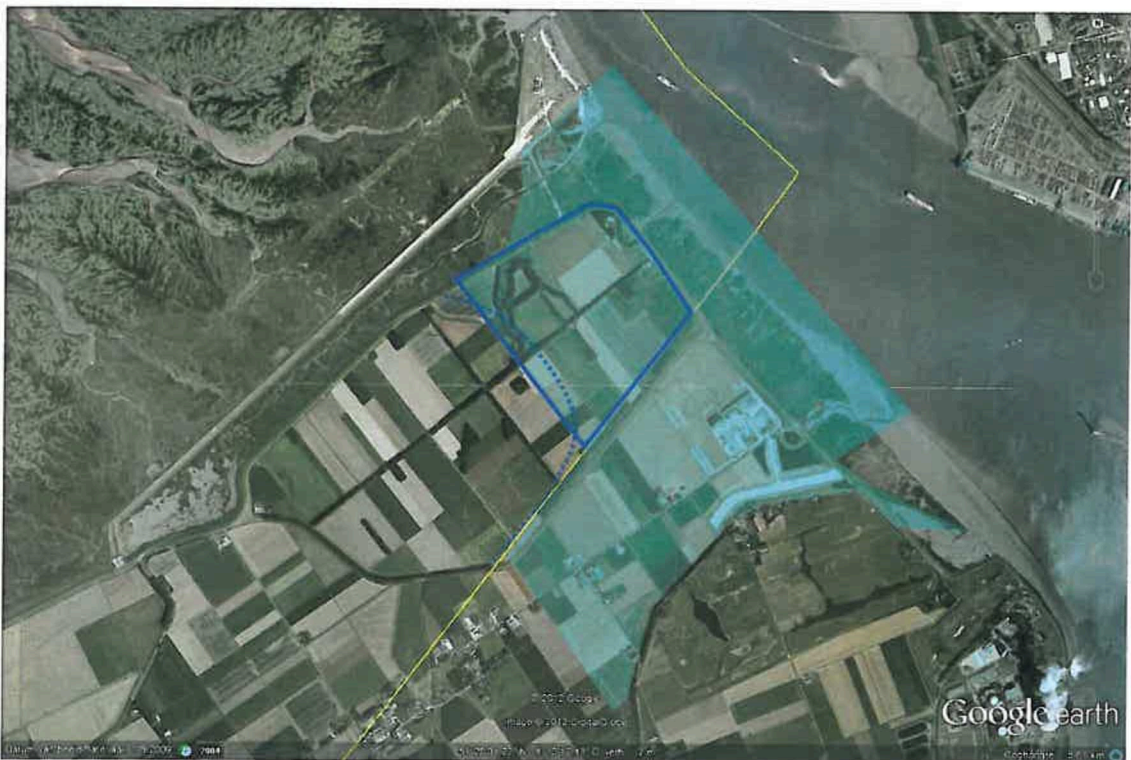
Tentative plan area for small Hedwige (dark blue line) polder and Prosper polder – a curved trajectory for the SW dike (dotted line) should be considered during the design
