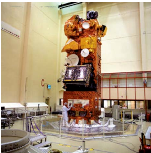
Figure 4: The Hydra Shaker tests satellites, but also large objects such as trains
