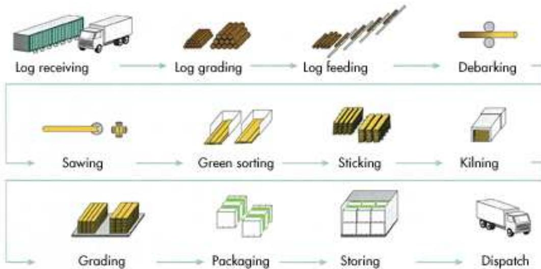
Figure 11: Overview of sawmill production process. Source: UPM<sup>124</sup>
