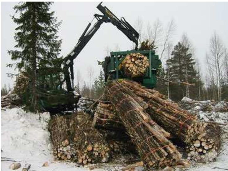
**Figure 10: Forest residue bundles and bundling machine.** Source: Northern Woodheat [Source: [http://elearn.ncp.fi/materiaali/kainulainens/nwh/woodfuel\\_supply\\_chains/forest\\_chips/bundling.htm](http://elearn.ncp.fi/materiaali/kainulainens/nwh/woodfuel_supply_chains/forest_chips/bundling.htm)]
