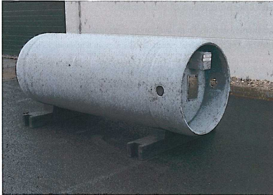
Figure 1-3 Standard 30B UF 6 cylinder
