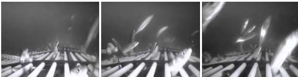
Figure 4.10. Camera footage from the gear adaptation with flexible tubes (the escape of a mackerel)
