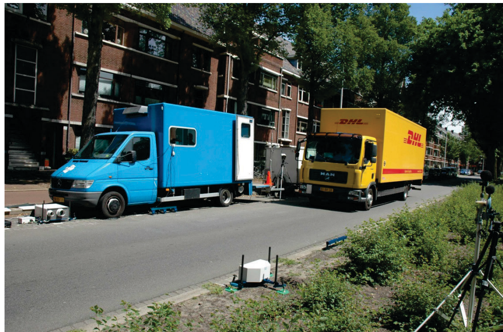
Figure 9: Schematic representation of the measurement set-up and a picture of the experimental set-up of Remote Emission Sensing in The Hague.
