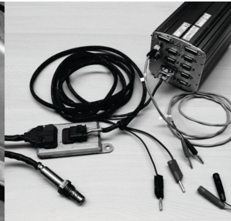
Figure 4: The sensor and data-acquisition unit which logs the sensor data, GPS data and optionally the CAN data.
