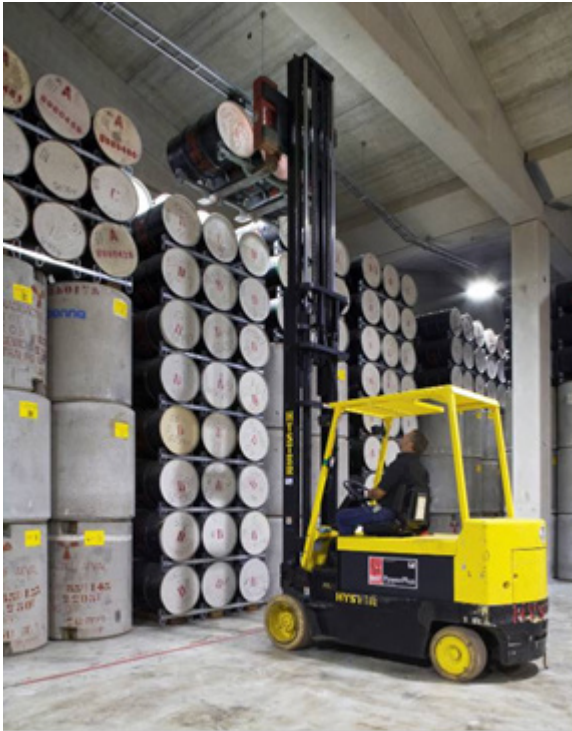
Figure A.2. The storage of low- and intermediate-level waste
