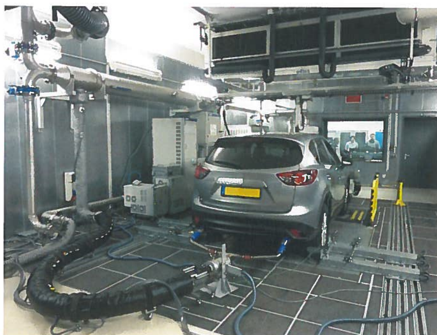
Figure 1: Emission test on a chassis dynamometer.
