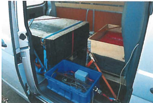
Figure 7: Load packages (the black box, left on the picture) and data logger of the SEMS (blue cradle).
