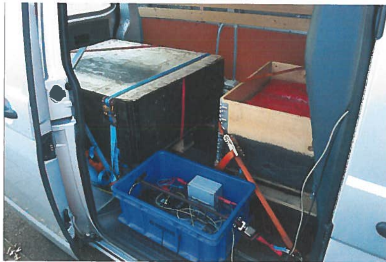
Figure 4: Load packages (black box) and data logger of the SEMS (blue cradle).
