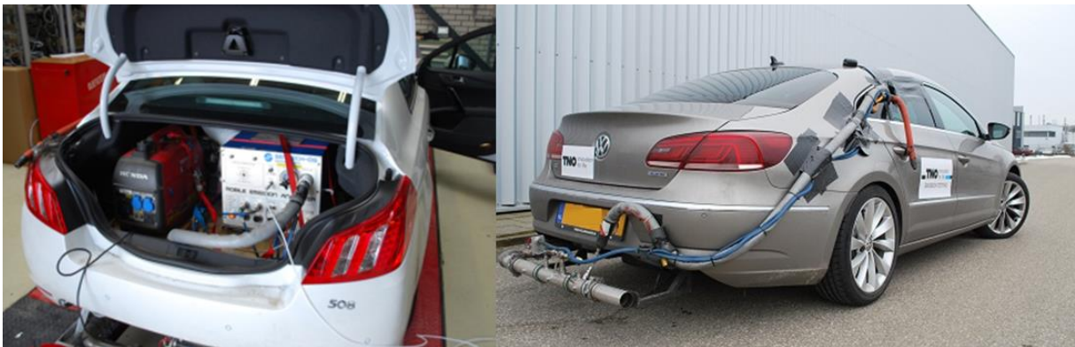
Figure 7: The PEMS system mounted on vehicles to be tested on the road
