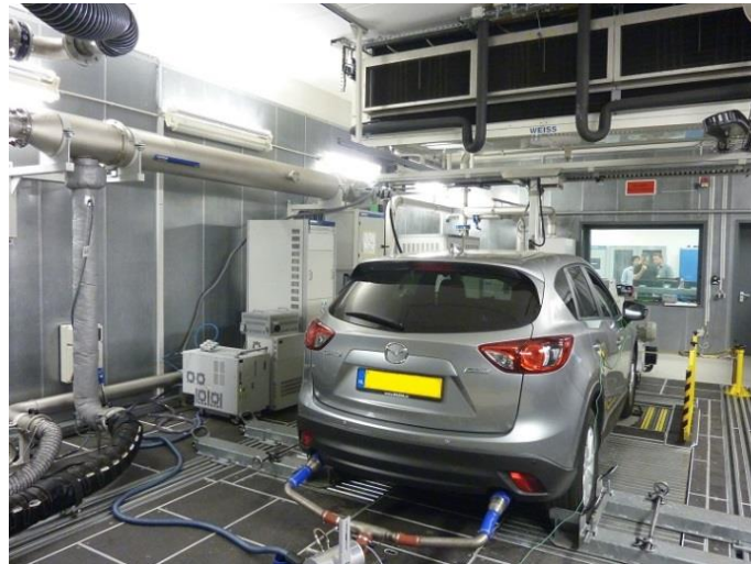
Figure 2: A passenger car tested in the laboratory on a two-wheel chassis dynamometer (roller bench)
