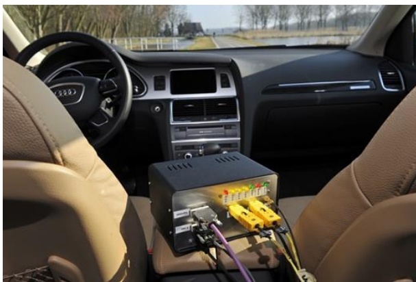
Figure 8: The SEMS system, developed by TNO, mounted on vehicles to be tested on the road (prototype version 2015)
