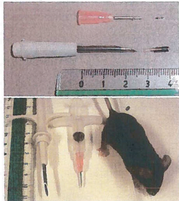
Figure 5 Size of microchips suited to mice (1 × 6 mm) and rats (2 × 12 mm) (top picture) and the size of the needles (12G, to the left and 18G, to the right) in relation to a fully grown C57BL mouse (bottom picture)
