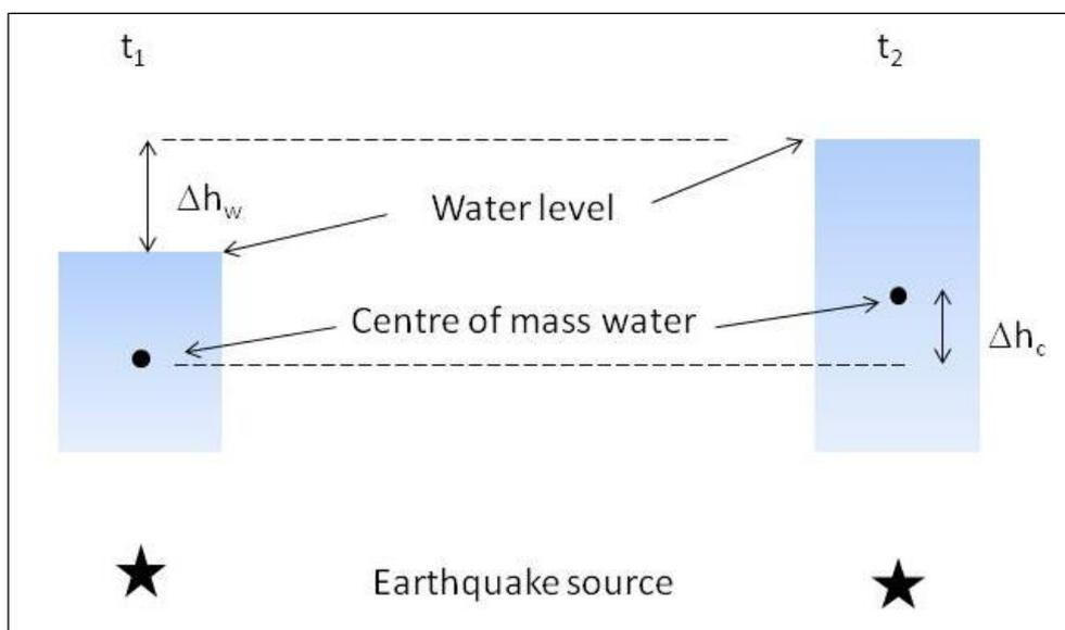
Fig. 38: Potential energy and water level rise
