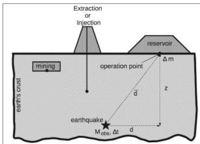
Fig. 36: Illustration of mass shift concept (KLOSE, 2013)
