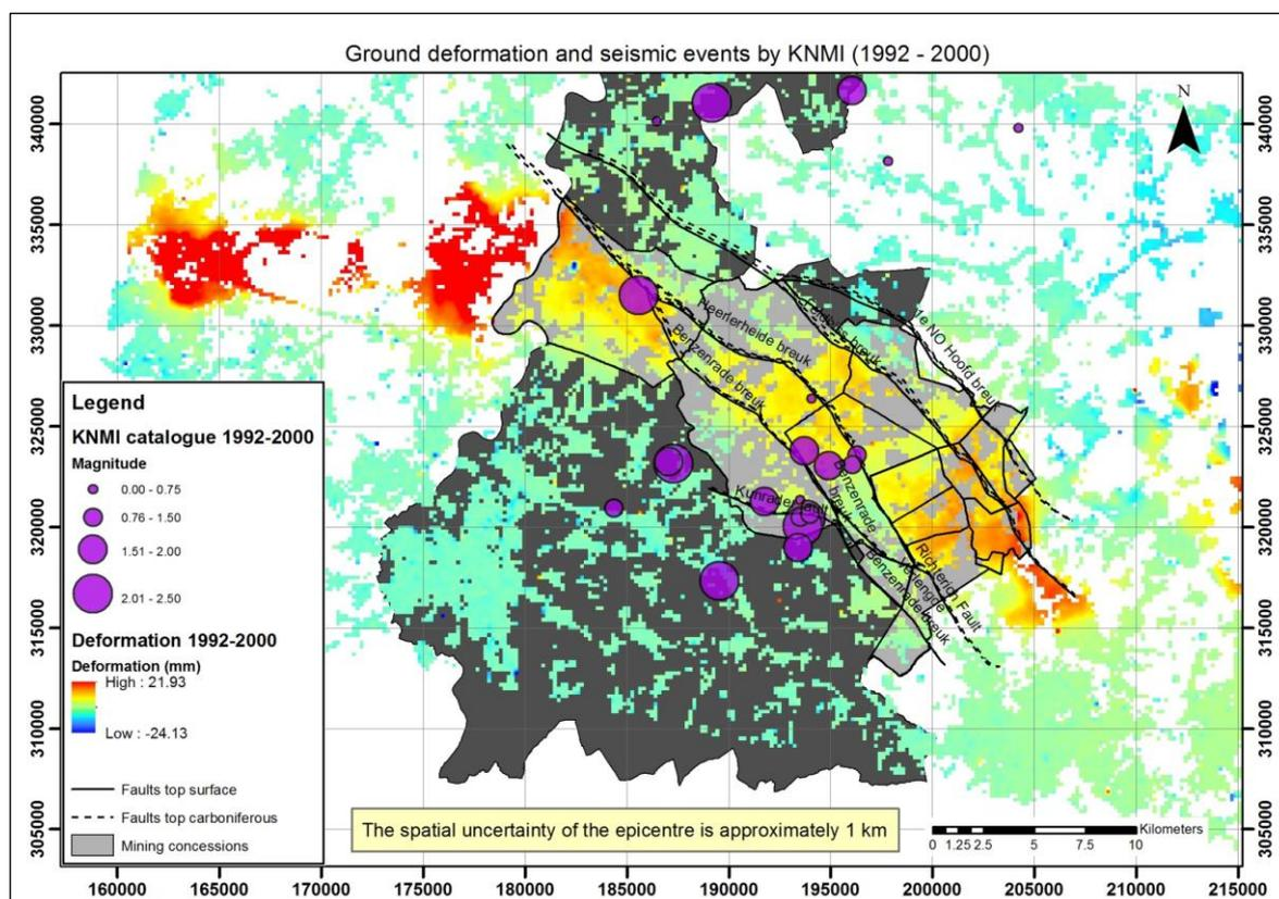
Fig. 23: Ground deformations from InSAR and seismic events 1992 - 2000
