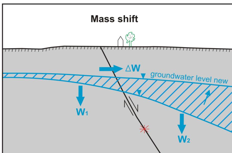
Fig. 4: Illustration of mass shift as triggering mechanism
