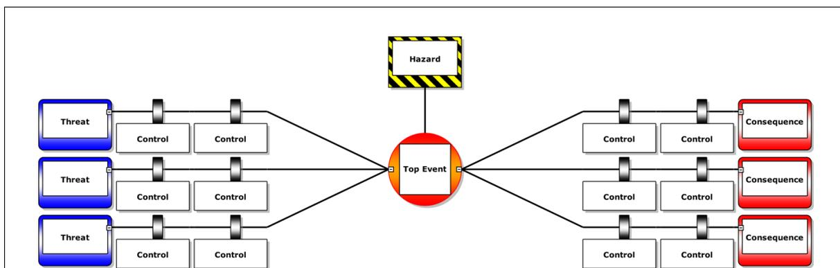
Fig. 5: Schematic representation of a Bow-Tie-Analysis
