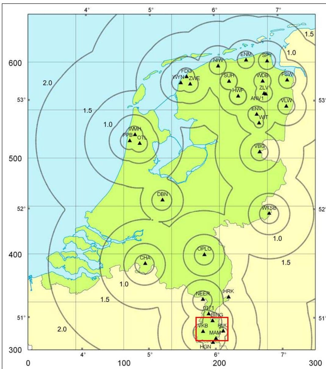
Fig. 14: Detection threshold during 2005 - 2010 (KNMI, 2012). The triangles show the seismic stations. The lines show the iso-magnitude threshold values. The area of interest is shown in the red box. Along the horizontal and vertical axes the coordinates (latitude and longitude are shown in degrees and distance is shown in kilometres)
