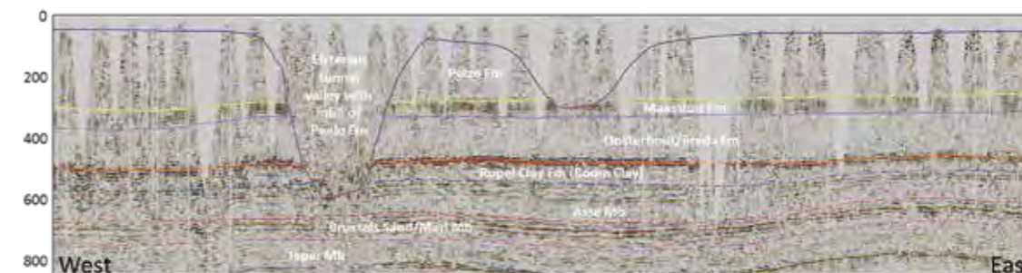
Figure 5-3-3: Seismic profile showing an Elsterian tunnel valley incised into the Boom Clay. The width of the section is ~25 km and depths are approximate [ten Veen, 2015: p.45].
