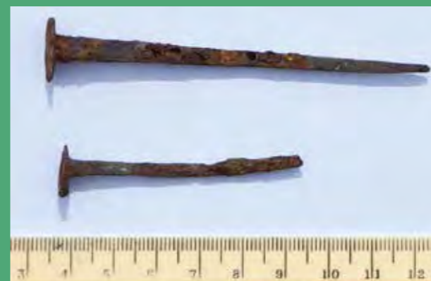
Above: Well-preserved Roman iron nails, about 2000 years old, from Inchtuthil, Scotland, showing limited superficial corrosion (scale: cm).
