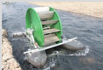
Barsha pump of aQysta at work
