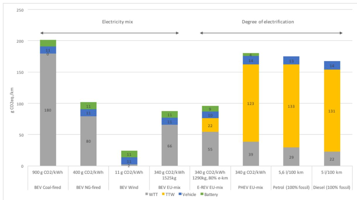
Figure 11 Impact of the electricity GHG footprint and the degree of electrification of the vehicle
