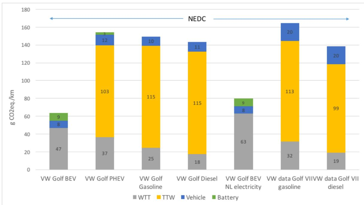
Figure 16 B “Apples and apples comparison” Comparison T31 VW Golf “NEDC” and VW data “NEDC”: in this comparison, the data as provided by VW are aligned with the T31 data, for the VW data the life time km is adapted to 252.000 km and the T31 model has calculated the NEDC GHG emissions. Please note that as mentioned the T31 model does not “optimize” the NEDC results as do OEMs
