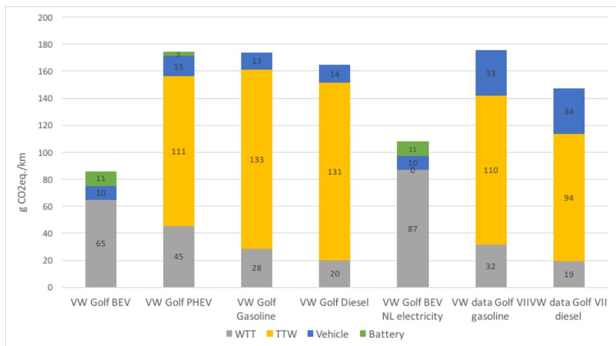
**Figure 16 A “Apples and pears comparison” VW Golf (generation VII) GHG LCA emissions per kilometer comparing T31 model and VW LCA calculations (“VW data”); the example is to show the current difficulty in comparing LCA data as published, please NOTE: the T31 and VW data cannot be compared 1 to 1: VW uses a 150.000 km used as LCA unit, T31 200.000 km life time; VW uses the NEDC test results, T31 the RDE emissions**
