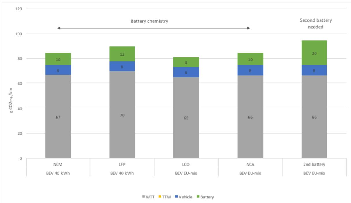
**Figure 9 Impact of the battery chemistry used on the life time GHG emissions. For all vehicles, a 40 kWh battery is being used and the electricity for charging the battery is in all cases EU-mix 2016. LCO has a very high cobalt content and is too expensive for EVs. Recycling is included in the impacts.**
