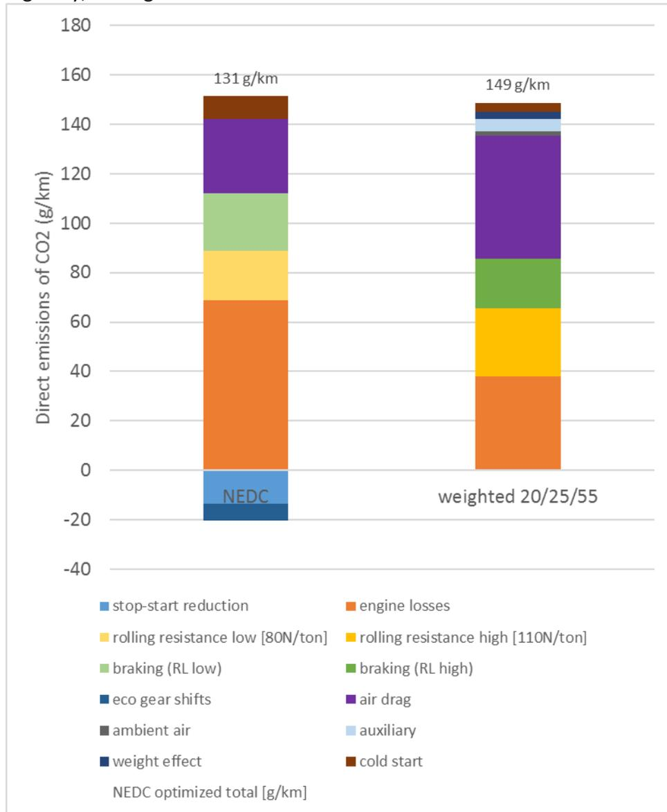
Figure 20 Example CO<sub>2</sub> emission breakdown for a 1250 kg 100 kW petrol car
