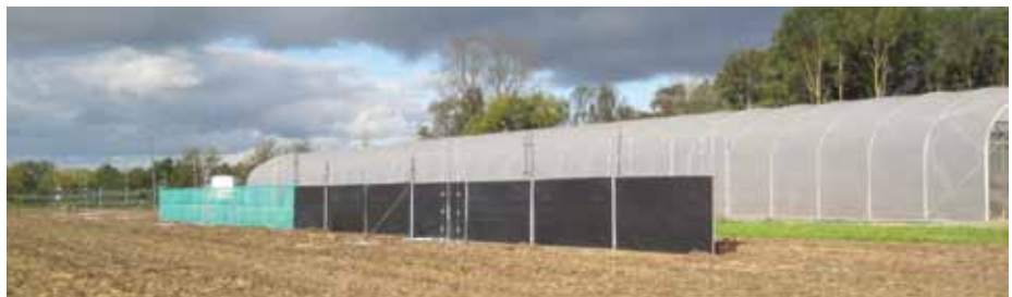
Figure 5.6: Overview of the measuring setup with a closed screen (D; black), permeable screen (C; light green) the open garden (B) and the full open space (A) in front of the tunnel with collectors in front and behind the screens.
