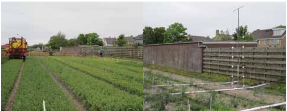
Figure 5.3: Overview of field layout of the spray drift measuring setup for the exposure of residents of flower bulb target field at a practical location (25 May 2016).
