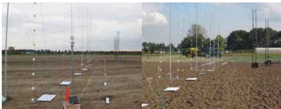
Figure 5.8: Spray drift measurement setup during experiments on the bare soil surface (left) and with the onion crop (right).
