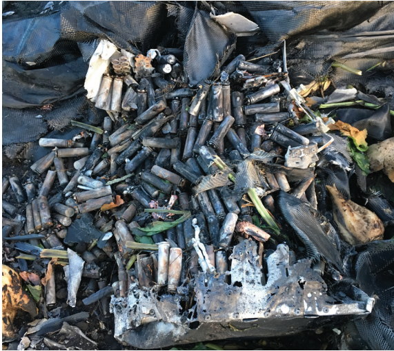
Figure 9: The burnt-out front battery pack.
