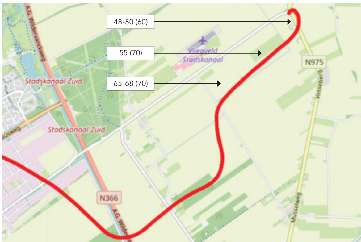
Figure 11: The last part of the flight; actual and prescribed (between brackets) airspeeds in knots. (Source: ATC the Netherlands and OpenStreepMap)
