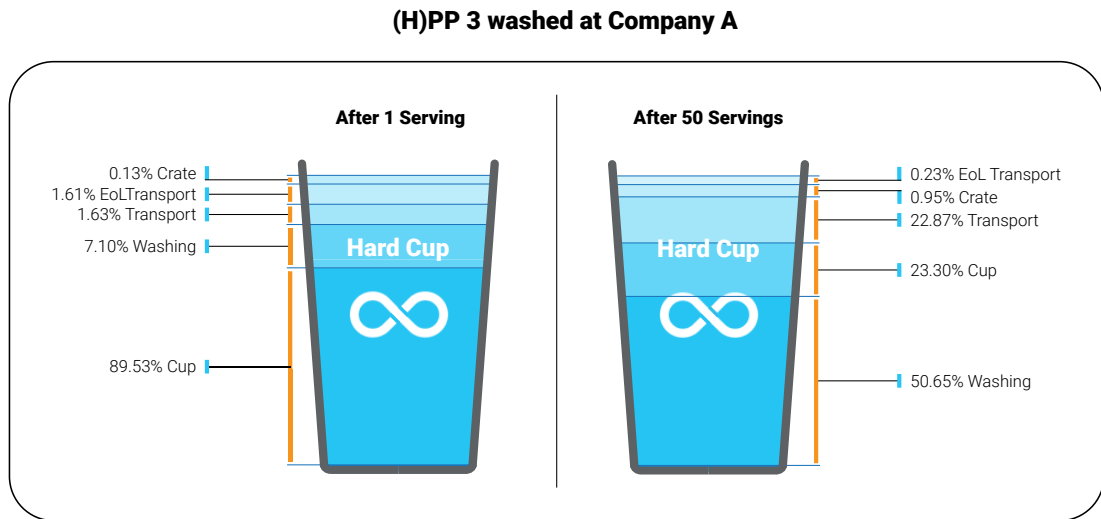
Figure 33: Comparison of 1 st and 50 th serving for most efficient Hard Cup systems
