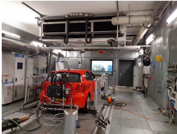
Figure 11-1: Validation of MEMS on the chassis dynamometer.
