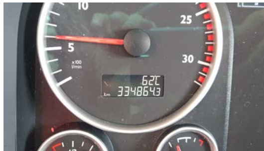
Figure 4: Photo of the display in the dashboard showing a value for the ambient temperature which deviates about 40 °C from the actual ambient temperature.
