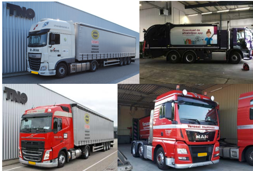
Figure 2: Tested vehicles with Euro VI step A to C certified diesel engines and one heavy-duty dual fuel engine (below left).
