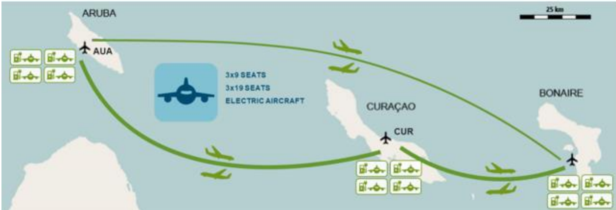
Figure 24: Overview of the pool of electric aircraft flying between the islands and the charging stations per airport
