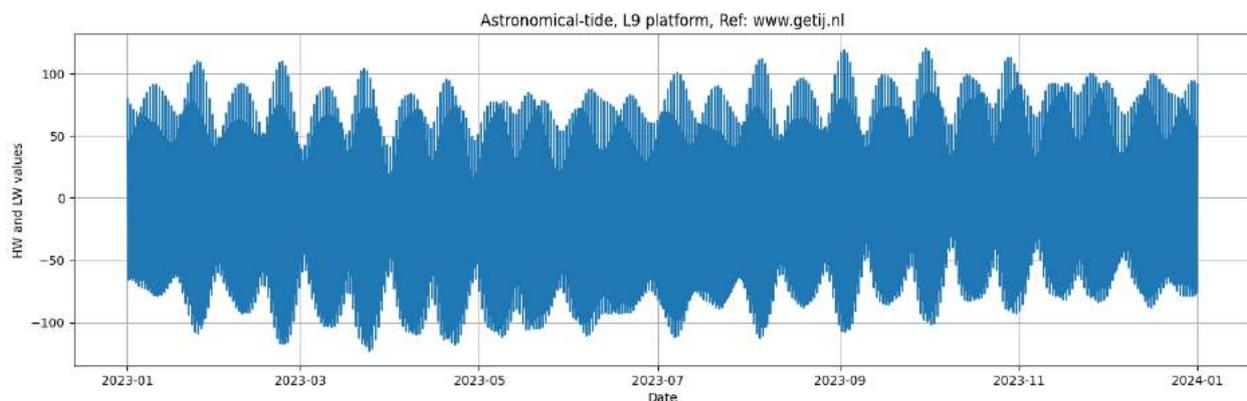
Figure 2-2: Astronomical tide prediction for 2023, platform L9 location.
