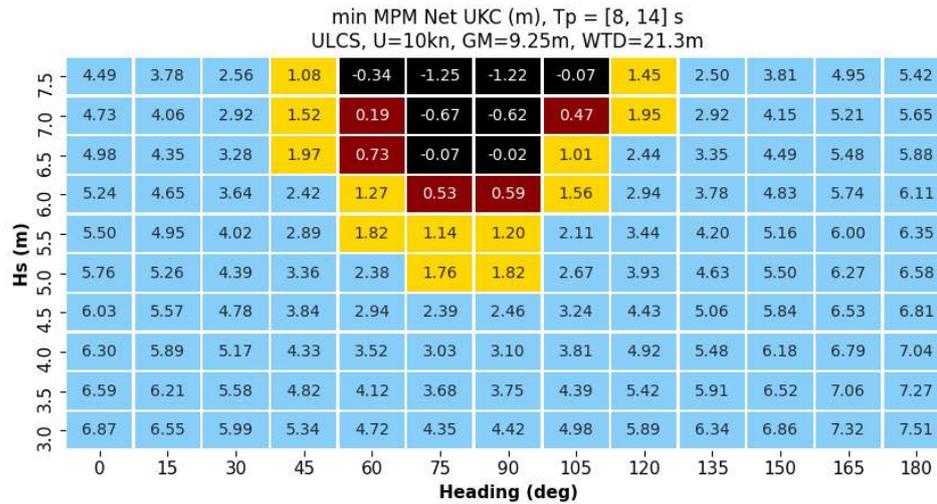
Net UKC taken at the hull sectional shape (to be used):
