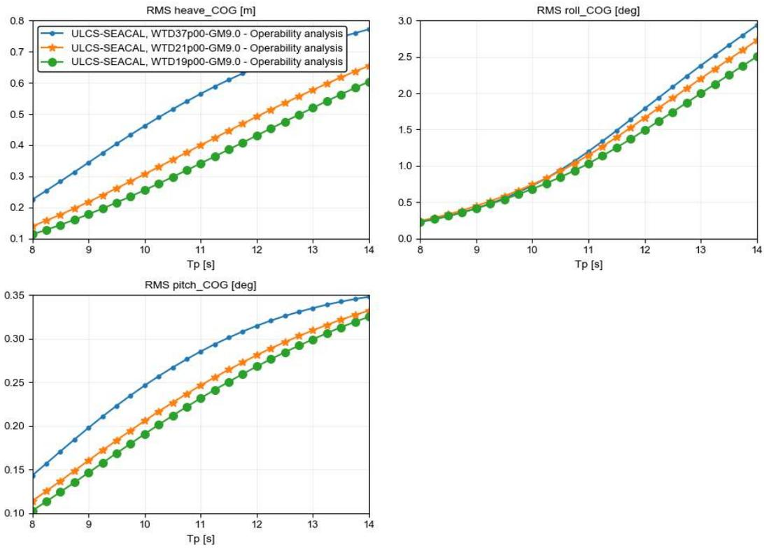
Figure 5-2: Global ship motions as function of water depth, Beam seas,  $H_s = 4.5$  m,  $T_m = 14.5$  m,  $GM = 9$  m.
