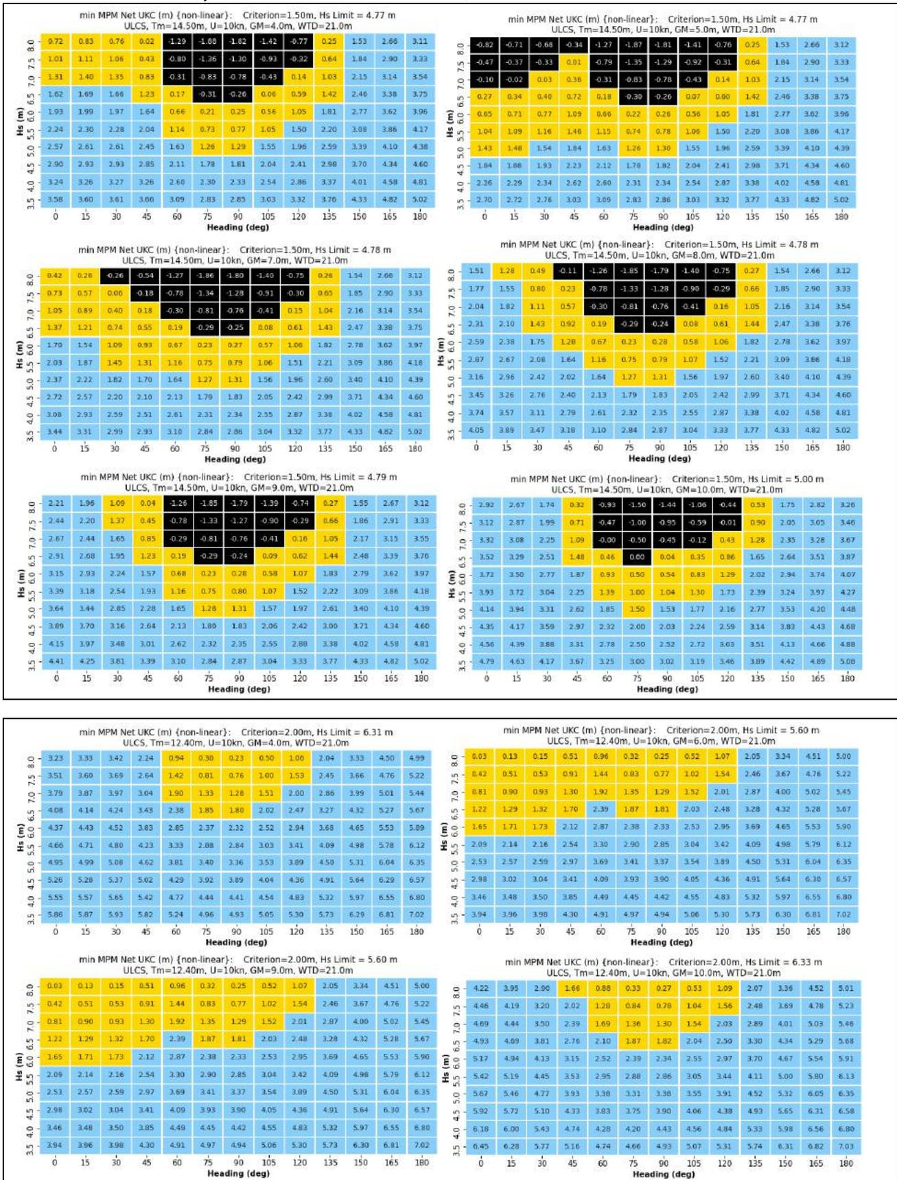
Table 5-8: MPM of dynamic under keel clearance, 19 m water depth, sailing draught 14.5 m and 12.4 m.
