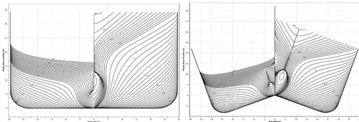
Figure 4-7: Hull lines of the ULCS, with zero heel and 20 deg heel (model split in aft and fwd part)
