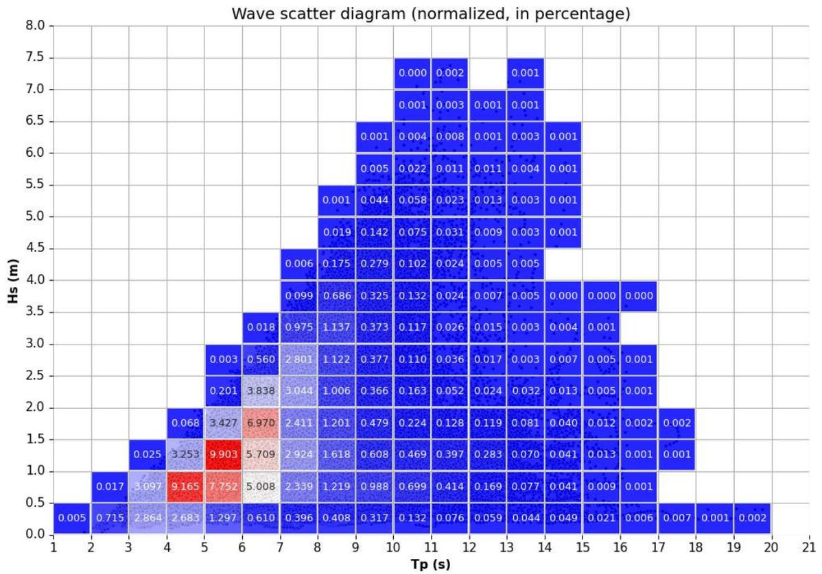
Figure 2-8: Normalised wave scatter diagram (40 years of data).
