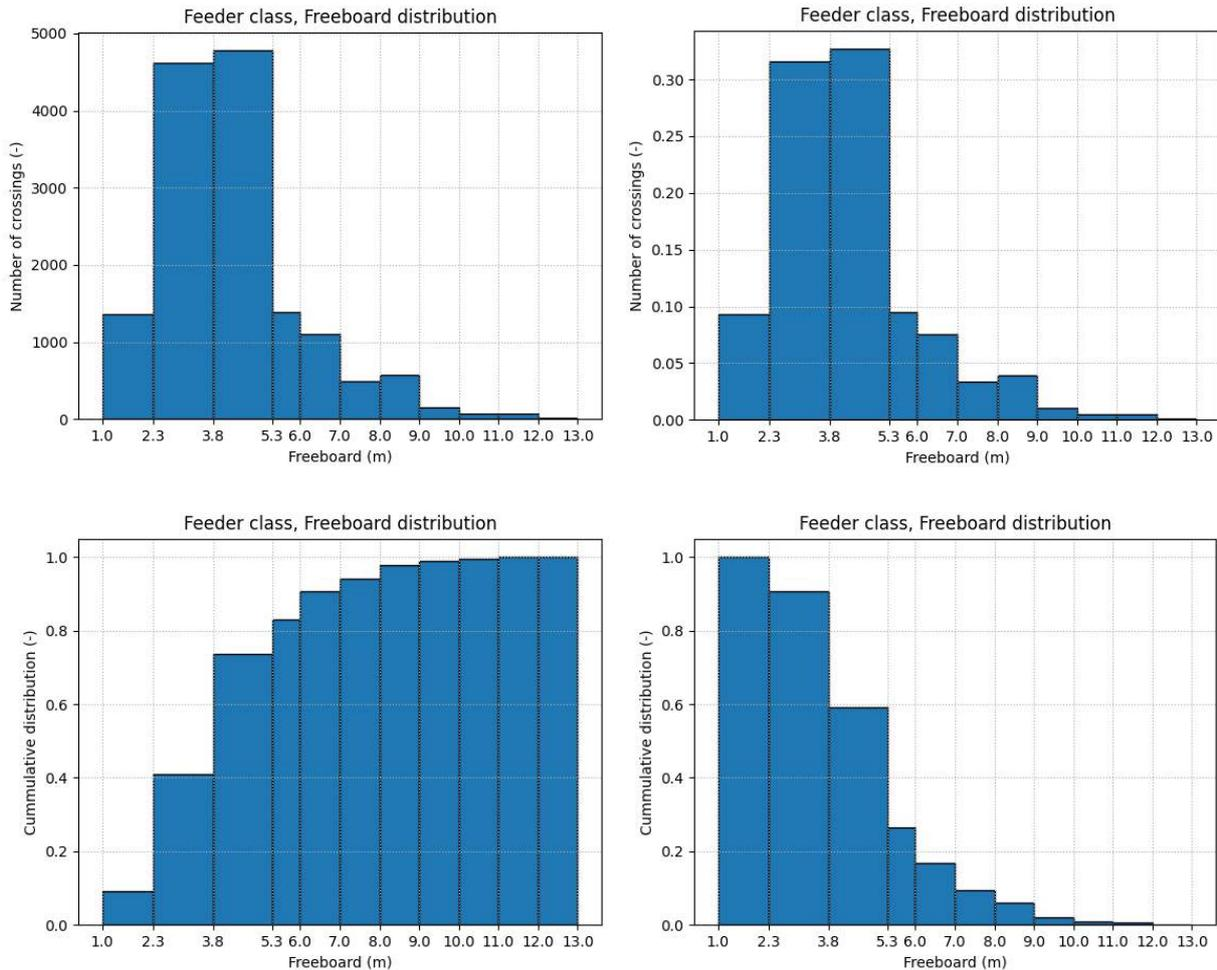
Figure 8-4: Actual freeboard height distribution of Feeder class; various presentations.
