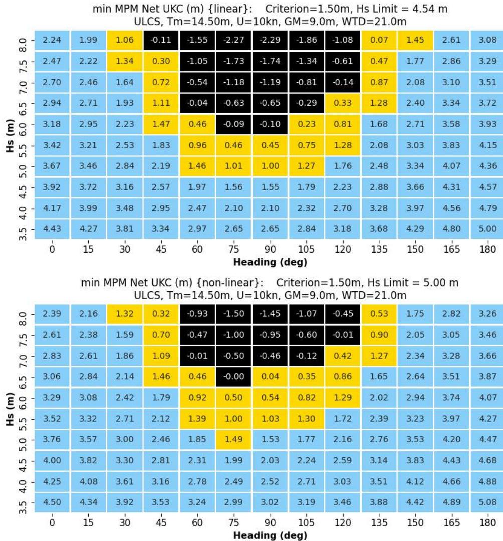
Figure 4-5: Dynamic UKC calculations for the ULCS without (top) and with (bottom) a correction for the shallow water kinematics in heave motion response.
