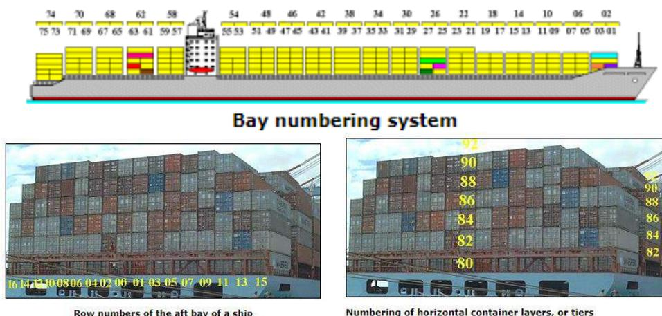
Figure 4-6: Container stowage reference system, bay-row-tier, from <https://www.containerhandbuch.de/>
