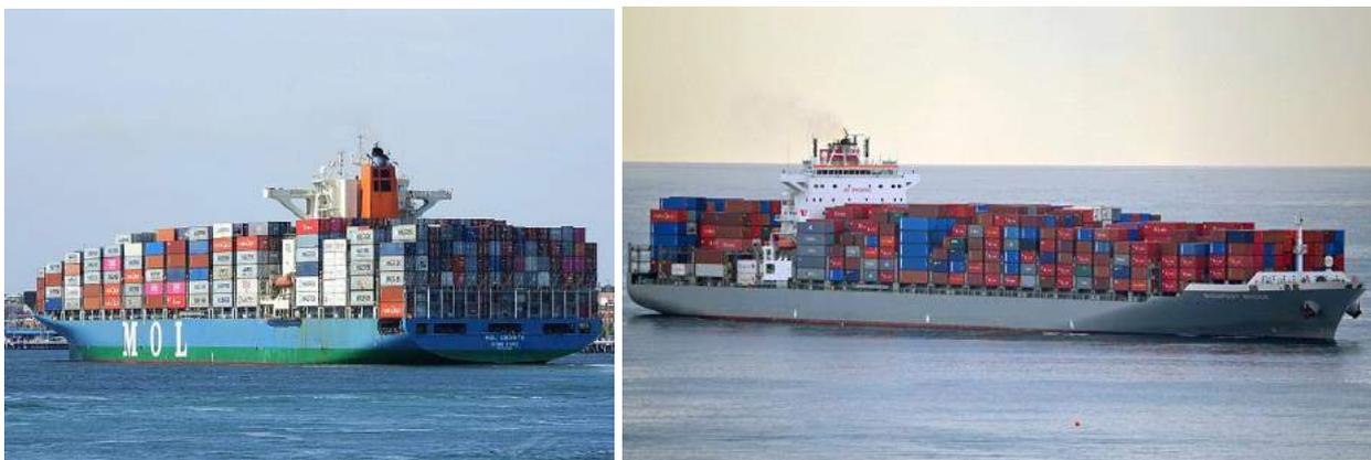
Figure 6-1: Typical Post-Panamax containerships with length < 297 m.
