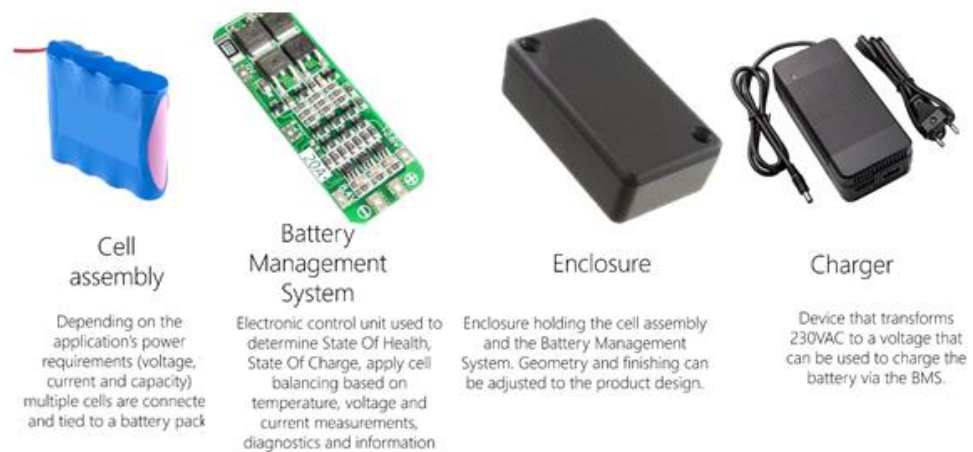
Figure 5-1: The battery pack and its main subcomponents as it will be considered in the assessment framework.
