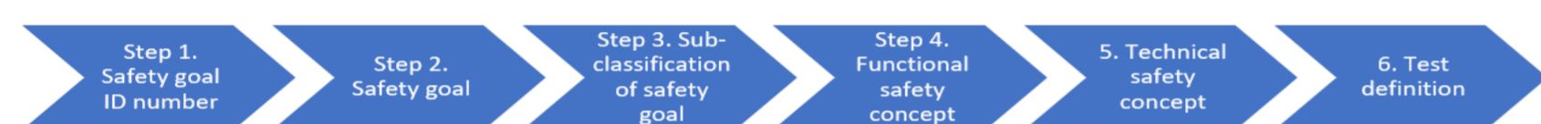
Figure 2: Safety goal definition, realisation and testing process.
