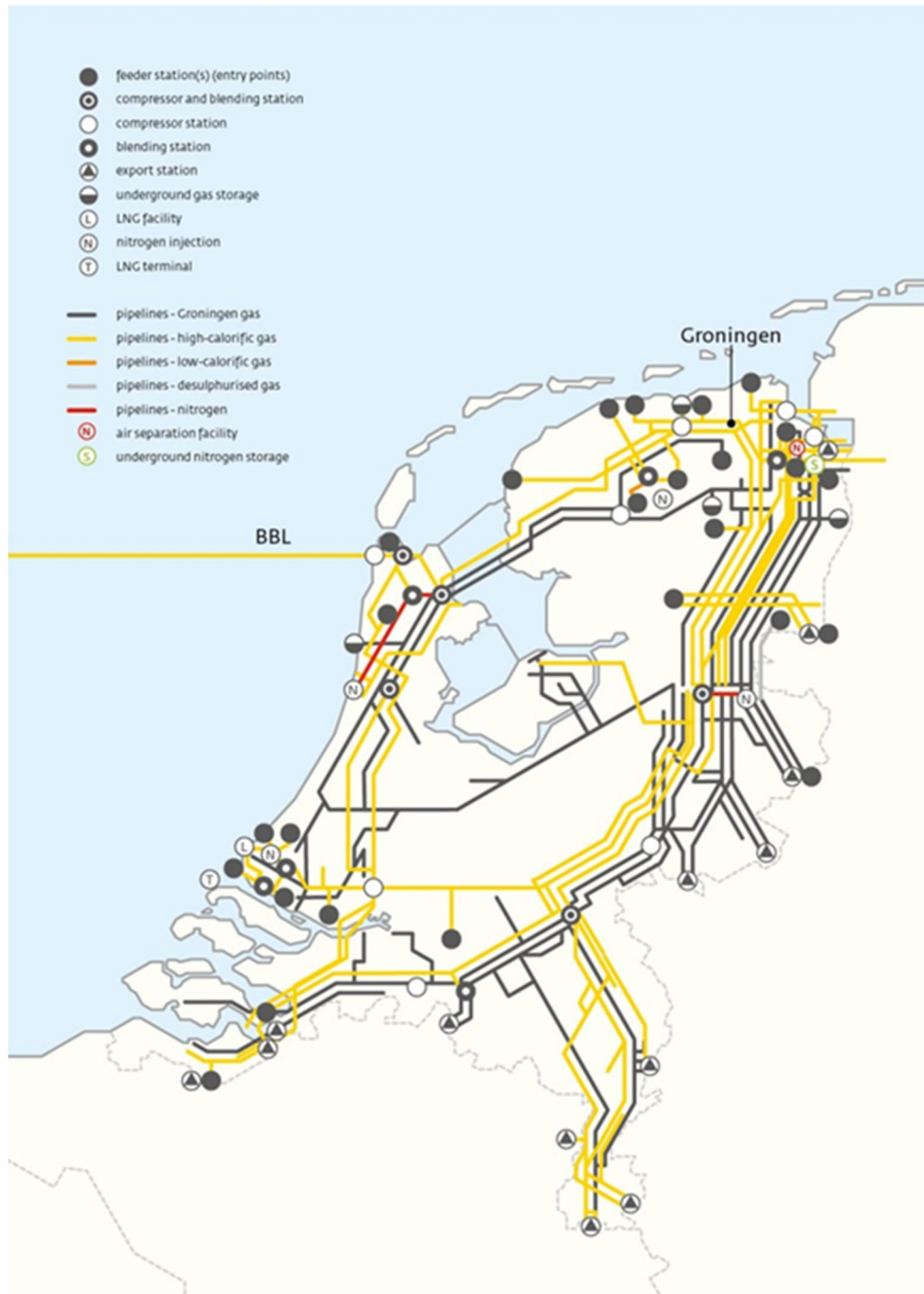
Figure 4: The high pressure gas network in the Netherlands. Source GTS
