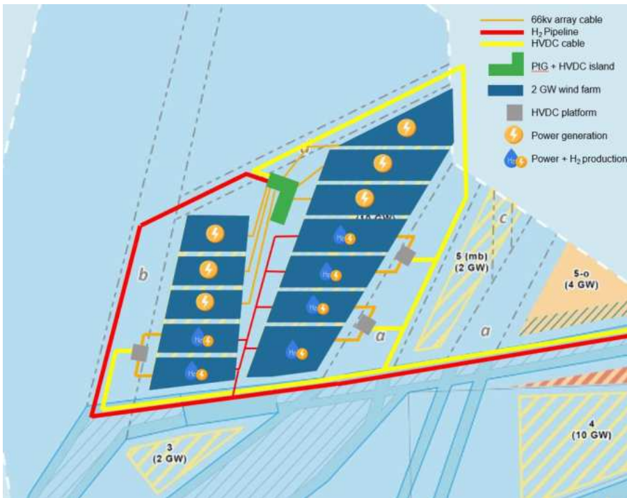
Figure 6.6: Illustrative Layout of Hybrid-based Energy Hub.
