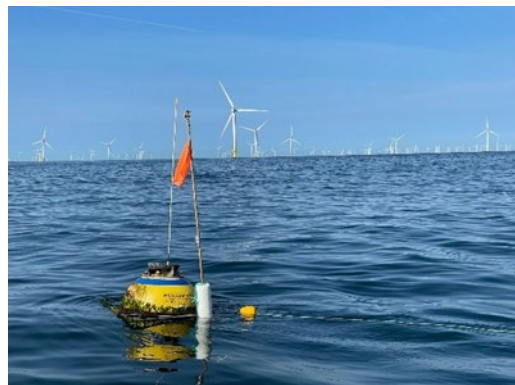
Figure A5.2: 24/05/2023 line of string F entwined with Rijkswaterstaat wave buoy
