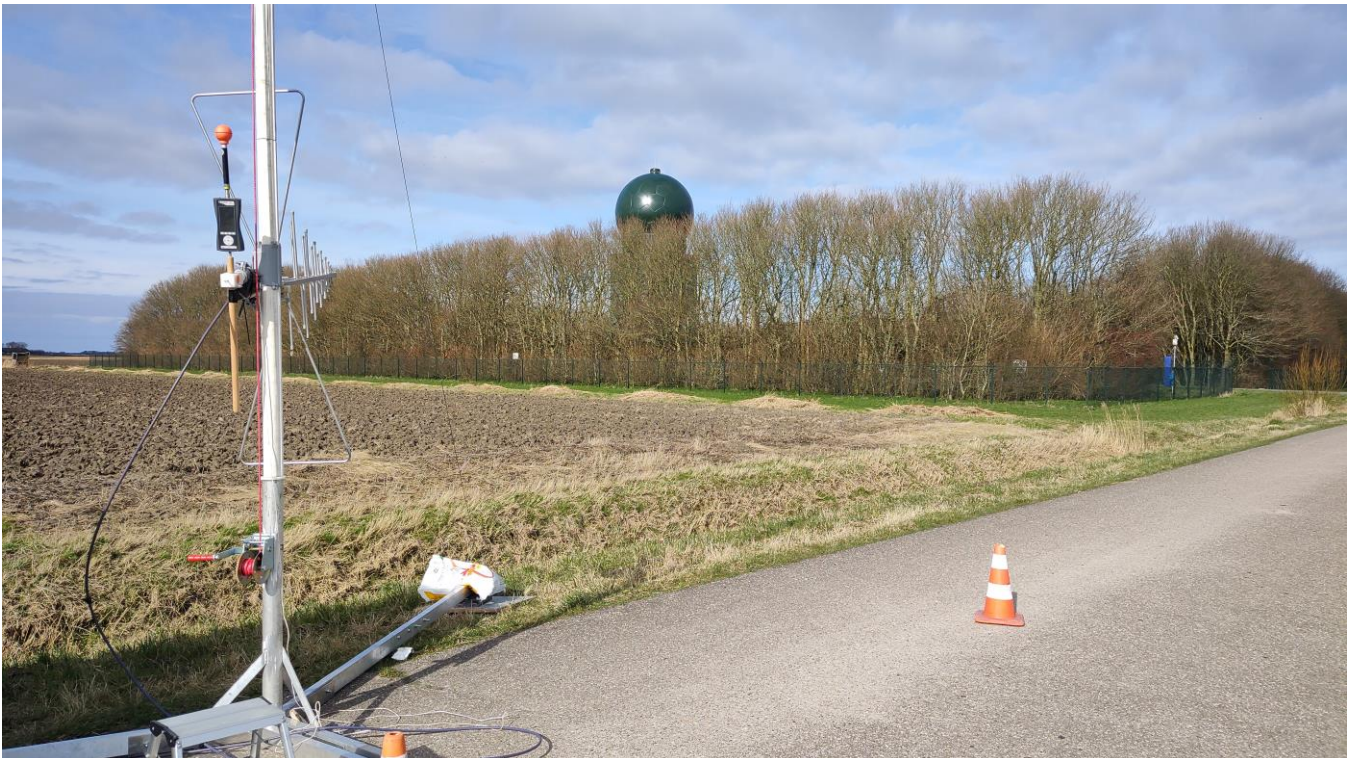
This photo shows the antenna position and height (2m) during ambient measurements performed below 1 GHz. At the frequency range above 1 GHz the antenna shown in section 1.5 (page 9) was used.
