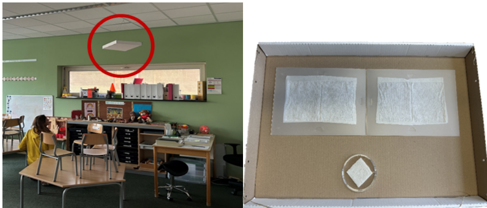
Figure C1: Left; a sampler box (in red circle) hanging in a classroom. Right; interior view of the cardboard box used for sampling containing an EDC (top) and a mini-EDC (bottom).
