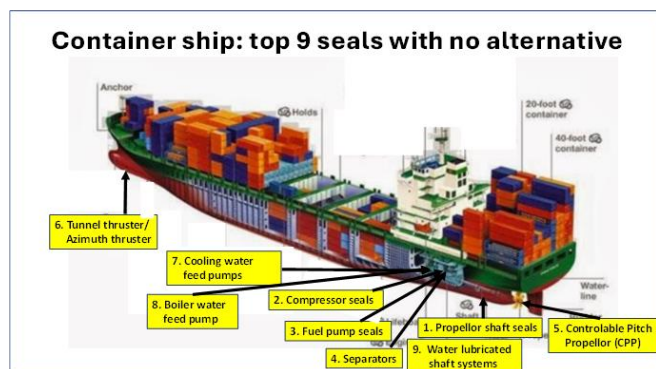
Container ship with (at least) 9 seals with no alternative material
